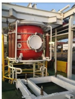
PDC CLOSED BELL IN THE HOOKS READY TO TRAVEL AWAY FROM MOONPOOL TOWARDS TUP CHAMBER
