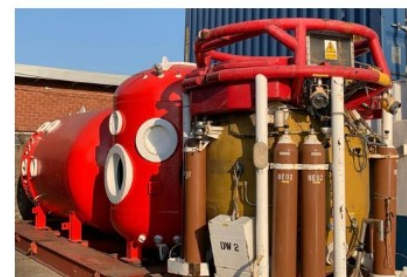
PDC SPARE SAT SYSTEM 3 THE DEEPEST SAT SYSTEM PDC HAS RATED TO 300 MSW (900FT) # MAN BELL WITH OSCULATING SIDE AND BOTTOM DOORS
