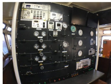
DEEPWORX DIVE CONTROL FOR THE PDC 3 MAN CLOSED BELL
