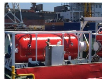
PDC SATURATION TWINLOCK CHAMBER CONSISTS OF LIVING CHAMBER AND WET POT (TUP) CHAMBER ALSO USED AS HRC WHICH PROVIDES MEANS FOR MEDICAL STAFF TO ENTER & EXIT ONCE RECOVERED TO LAND FROM TOWING OPERATION. THIS TWIN LOCK HRC ELIMINATES THE NEED FOR A HRC IN TRAINING
