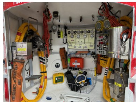
INSIDE THE PDC CLASSROOM TRAINING AID BELL AN EXACT COPY OF THE PDC 3 MAN OPERATIONAL CLOSED BELL
